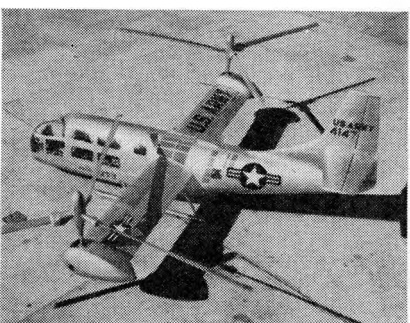
20 A new-type plane with tilting rotors is: (a) an amphibian (c) a helioplane (b) an autogiro (d) a convertiplane
